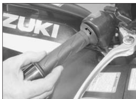
7.3 Twist the throttle and measure the amount of free rotation
