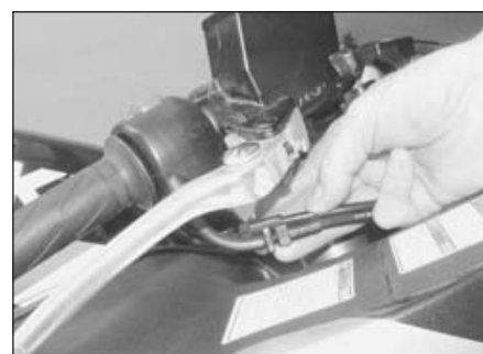
7.4 Slacken the adjuster lockrings and turn the adjusters as described
