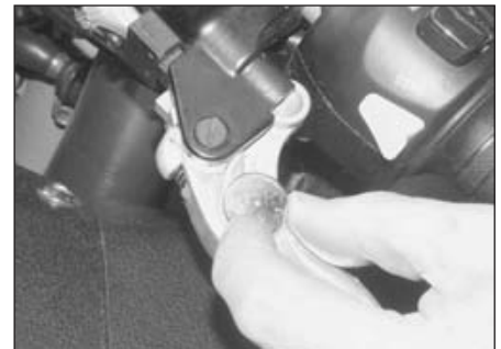
8.6 Clutch lever span adjuster – align the required setting number with the arrow on the lever
