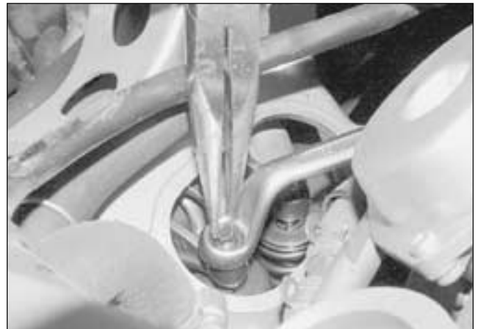
16.7b Slacken the locknut using an offset ring spanner and turn the adjusting screw using pliers
