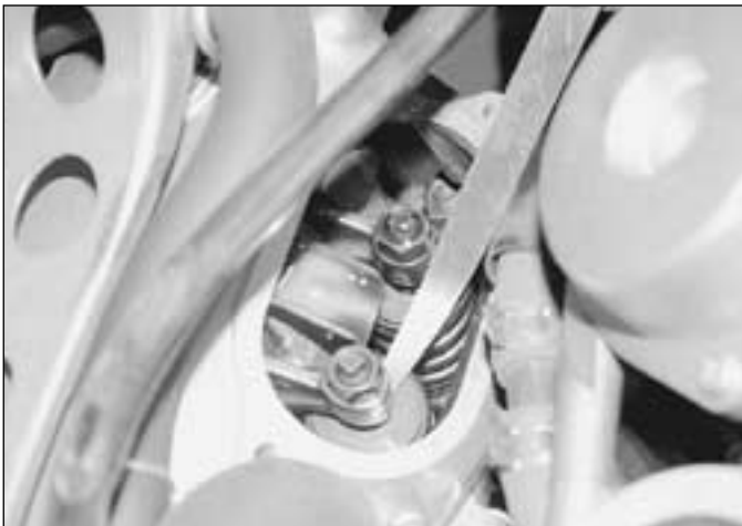
16.7a Insert the feeler gauge between the base of the adjusting screw and the top of the valve stem as shown
